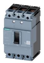
circuit breaker 3VM1 IEC frame 100 breaking capacity class N Icu=25kA @ 415V 3-pole, line protection TM210, FTFM, In=80A overload protection Ir=80A, not adjustable short-circuit protection Ii=10 x In nut keeper kit
