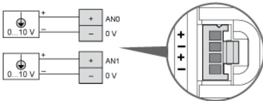
The (-) poles are connected internally.
