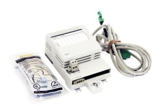
External DIN-rail mounted rechargeable battery unit for AC 800M controllers, including lithium-ion battery, 24V DC connector and connection cable TK821V020. Width=85 mm. Equivalent amount of Lithium metal=0,8g (0,03oz)
