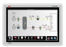
Touchscreen panels with brilliant TFT/LED display colors and multiprotocol connectivity. The standard range of Panel 800 comprises of PP875, PP881, PP883, PP886 and PP895 that are easy-to use HMI with comprehensive and integrated templates and libraries for every conceivable process you need. All standard panels are equipped with high-resolution graphics in TFT/LED display. Most models offer wide screen, high resolution display for increased efficiency and excellent operator interaction.
