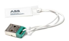
Panel 800 Runtime and dedicated license dongles, makes Panel 800 applications to be run on normal Windows PC. This enables engineering efficient reuse of the panels applications in situations when a PC based HMI is required in addition to process panels.
