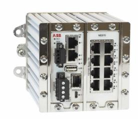
NE870 is an industrial router which also acts as a firewall. The router/firewall can be utilized to segment a system in to network areas and also security zones. NE870 is primarily intended to be used to separate client/server networks and control networks, to separate different control and safety networks, but also to create RNRP tunnel areas between RNRP networks.
