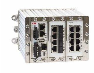
NE820 is an Industrial switch made for harsh environments. The switch can be used in either 100 Mbit or Gigabit networks due to our multi-rate SFP solution. Our unique FRNT (Fast Recovery of Network Topology) technology is the fastest protocol on the market to reconfigure a network in the event of any link or hardware failure. That is why NE820 is also used in safety critical applications such as tunnels, traffic signal control and railway systems.
