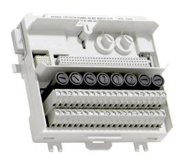
The TU838 MTU can have up to 16 I/O channels. The maximum rated voltage is 50 V and maximum rated current is 3 A per channel. The MTU distributes the ModuleBus to the I/O module and to the next MTU. It also generates the correct address to the I/O module by shifting the outgoing position signals to the next MTU.
