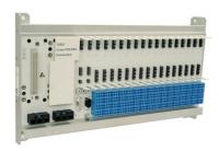
The remote S900 I/O system can be installed in non-hazardous areas or directly in Zone 1 or Zone 2 hazardous area depending on the selected system variant. S900 I/O communicates with the control system level using the PROFIBUS DP standard. The I/O system can be installed directly in the field, therefore the costs for marshalling and wiring are reduced.
