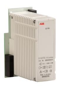
The remote S900 I/O system can be installed in non-hazardous areas or directly in Zone 1 or Zone 2 hazardous area depending on the selected system variant. S900 I/O communicates with the control system level using the PROFIBUS DP standard. The I/O system can be installed directly in the field, therefore the costs for marshalling and wiring are reduced.
