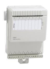
The DI803 is an 8 channel 230 V a.c./d.c. digital input module for the S800 I/O. This module has 8 digital inputs. The a.c. input voltage range is 164 - 264 volt and the input current is 7.6 mA at 230 V a.c. The d.c. input range is 175 - 275 V and the input current is 1.6 mA at 220 V. The inputs are individually isolated. Every input channel consists of current limiting components, EMC protection components, input state indication LED and optical isolation barrier.
