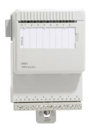
The DI802 is an 8 channel 120 V a.c./d.c. digital input module for the S800 I/O. This module has 8 digital inputs. The a.c. input voltage range is 77 - 130 volt and the input current is 10 mA at 120 V a.c. The d.c. input range is 75 - 145 V and the input current is 2.8 mA at 110 V. The inputs are individually isolated. Every input channel consists of current limiting components, EMC protection components, input state indication LED and optical isolation barrier.
