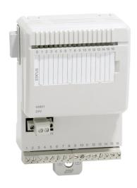
The DI801 is a 16 channel 24 V digital input module for the S800 I/O. This module has 16 digital inputs. The input voltage range is 18 to 30 volt d.c. and the input current is 6 mA at 24 V. The inputs are in one isolated group with sixteen channels and channel number sixteen can be used for voltage supervision input in the group. Every input channel consists of current limiting components, EMC protection components, input state indication LED and optical isolation barrier.
