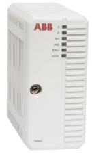
S800 I/O is a comprehensive, distributed and modular process I/O system that communicates with parent controllers and PLCs over industry-standard field buses. The TB840 ModuleBus Modem is a fiber optic interface to the Optical ModuleBus. TB840A is used in redundancy configurations where each module is connected to different optical ModuleBus lines, but connected to the same electrical ModuleBus.
