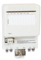
S800 I/O is a comprehensive. distributed and modular process I/O system that communicates with parent controllers and PLCs over industry-standard field buses. The TB825 ModuleBus Optical media converter, converts between plastic opto fiber or HCS fiber with versatile link connectors and glass optical fiber with ST connetcors.
