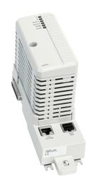
The CI874 is an AC 800M communication interface that connects to external Ethernet devices using the OPC UA protocol. The TP867 Baseplate has one RJ45 Ethernet connector that supports 100Mbps. The CI874 expansion unit contains the CEX-Bus logic, a communication unit, and a DC/DC converter that supplies the required voltage from  $\pm 24$  V supply through the CEX-Bus.
