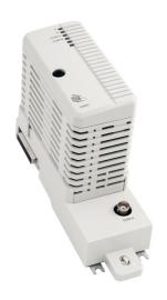
The CI865 module is the AC 800M system's communication interface for Satt ControlNet and bridges different bus standards used on AC 800M and Satt ControlNet. The CI865 module makes it possible to use older Satt I/O system (Rack I/O and Series 200 I/O) with the AC 800M controller platform, but it cannot be used as a general ControlNet interface. CI865 cannot be used in a High Integrity controller.
