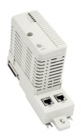
The MasterBus 300 (MB300) communication protocol used in communication between controllers, operator stations in installations based on Advant OCS with Master software is also implemented in the System 800xA controller AC 800M. MB 300 communication is realized in AC 800M by communication interface CI855, which is connected to the CEX-Bus through a baseplate.
