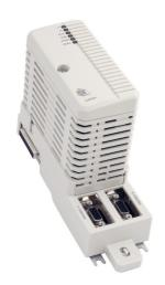
PROFIBUS DP is a high speed multipurpose bus protocol (up to 12Mbit/s) for interconnecting field devices, like remote I/O, drives, low voltage electrical equipment, and controllers. PROFIBUS DP can be connected to the AC 800M via the CI854B communication interface. The CI854B includes two PROFIBUS ports to realize line redundancy and it also supports PROFIBUS master redundancy.
