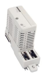
PROFIBUS DP is a high speed multipurpose bus protocol (up to 12Mbit/s) for interconnecting field devices, like remote I/O, drives, low voltage electrical equipment, and controllers. PROFIBUS DP can be connected to the AC 800M via the CI854A communication interface. The Classic CI854A includes two PROFIBUS ports to realize line redundancy and it also supports PROFIBUS master redundancy. The CI854B is the new PROFIBUS-DP master that replaces CI854A in new installations.
