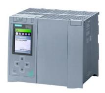
SIMATIC S7-1500T, CPU 1516T-3 PN/DP, Central processing unit with 1.5 MB RAM for program and 5 MB for data, 1st interface: PROFINET IRT with 2-port switch, 2nd interface, Ethernet, 3rd interface, PROFIBUS, 10 ns bit performance, SIMATIC Memory Card required
