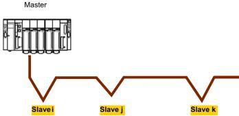
Only one device can transmit on the line at any time. The master manages the exchanges and only it can take the initiative.
