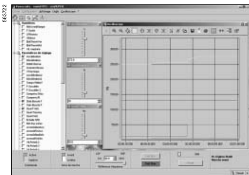
Monitoring the different parameters with the oscilloscope function in PowerSuite for PC
