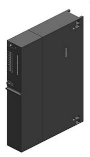
SIPLUS S7-400 CPU 417-4 -25 ... +70°C with conformal coating based on 6ES7417-4XT07-0AB0. Central processing unit with: "Work memory 32 MB, (16 MB code;" 16 MB data) Interfaces 1st "interface MPI 12 Mbit/s; 2nd" interface PROFIBUS DP, 3rd/4th interface plugin IFM module
