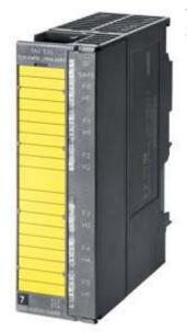
SIPLUS S7-300 SM336 F 6AI 15 bit -25...+60 °C (70 °C with forced convection) With conformal coating Based on 6ES7336-4GE00-0AB0 . Fail-safe analog inputs For SIMATIC Safety, with HART support, up to Category 4 (EN 954-1) /SIL3 (IEC 61508)/ PLE (ISO 13849), 1x 20-pole
