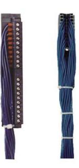
S7-300 FRONT CON. W. SINGLE COR. 3.2 M Front connector for SIMATIC S7-300 20 pole (6ES7392-1AJ00-0AA0) with 20 single cores 0.5 mm2, Single cores H05V-K, Screw version VPE=5 units L = 3.2 m
