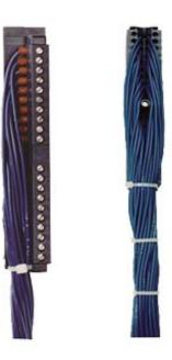
S7-300 FRONT CON. W SINGLE COR. 3.2 M UL Front connector for SIMATIC S7-300 20 pole (6ES7392-1AJ00-0AA0) with 20 single cores AWG 20, Single cores UL / CSA AWM Style 1007/1569 FT2 TR64 Screw version VPE=1 unit L = 3.2 m
