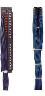
S7-300 FRONT CON. W. SINGLE CO  $2.5 \, \text{M}$ Front connector for SIMATIC S7-300 40 pole (6ES7392-1AM00-0AA0) with 40 single cores 0.5 mm2, Single cores H05V-K, Screw version VPE=5 units L =  $2.5 \, \text{m}$
