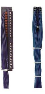
S7-300 FRONTCON. SINGLE CO 2.5 M CRIMP Front connector for SIMATIC S7-300 40 pole (6ES7921-3AH20-0AA0) with 40 single cores 0.5 mm2, Single cores H05V-K, Crimp version VPE=1 unit L = 2.5 m
