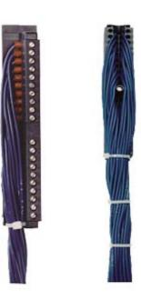
S7-300 FRONT CONN. W. SINGLE CORE  $\,2.5\,\mathrm{M}$  Front connector for SIMATIC S7-300 40 pole (6ES7392-1AM00-0AA0) with 40 single cores 0.5 mm2, Single cores H05V-K, Screw version VPE=1 unit L =  $2.5\,\mathrm{m}$
