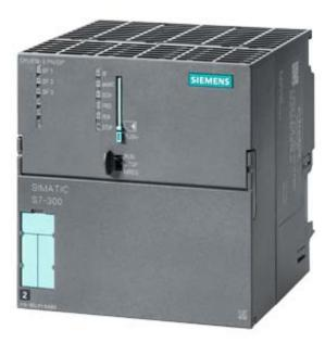
SIMATIC S7-300 CPU 319-3 PN/DP, Central processing unit with 2 MB work memory, 1st interface MPI/DP 12 Mbit/s, 2nd interface DP master/slave 3rd interface Ethernet PROFINET, with 2-port switch, Micro Memory Card required
