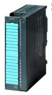
SIPLUS S7-300 SM 332 4AO with conformal coating based on 6ES7332-7ND02-0AB0 . Analog output isolated by channel, 4 AI, Resolution 16 bit, 0-10 V, 1-5 V, +/-10 V, +/-20 mA, 0/4-20mA, 20pole, suitable for isochronous mode operation improved bus cycle times for+ the isochronous mode
