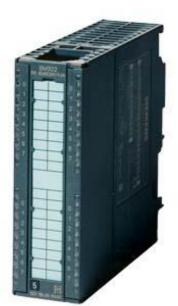
SIPLUS S7-300 SM 322-40-pole -25...+60 °C With conformal coating based on 6ES7322-1HF10-0AA0 . Digital output Isolated 8 DQ (relay), 1x 40-pole, 24 V DC, 5 A or 230 V AC, 5 A, connectors with spring-loaded terminal can be used as of 6ES7392-1BM01-0AA0
