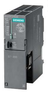
SIPLUS S7-300 CPU 317F-2PN/DP conformity with EN 50155 T1 Kat 1 Kl A/B based on 6ES7317-2FK14-0AB0 . Central processing unit with 1.5 MB work memory, 1st interface MPI/DP 12Mbit/ s, 2nd interface Ethernet PROFINET, with 2-port switch, Micro Memory Card required
