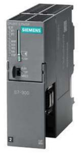
SIPLUS S7-300 CPU 317-2PN/DP -25...+60°C Conformity with EN 50155 T1 Kat 1 KI A/B with conformal coating based on 6ES7317-2Ek14-0AB0 . Central processing unit with 1 MB work memory, 1st interface MPI/DP 12Mbit/ s, 2nd interface Ethernet PROFINET, with 2-port switch, Micro Memory Card required
