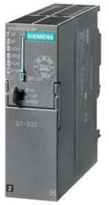
SIPLUS S7-300 CPU 315F-2DP with conformal coating according to EN 50155 T1 Cat 1 Cl A/ B based on 6ES7315-6FF04-0ab0 . Fail-safe module with MPI Integr. power supply 24 V DC, Work memory 384 KB, 40 mm width, 2nd interface DP master/ slave Micro Memory Card required
