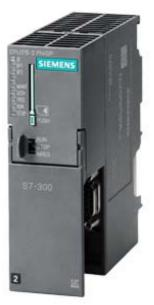
SIPLUS S7-300 CPU 315F-2PN/DP -25...+60°C with conformal coating based on 6ES7315-2FJ14-0AB0 . Central processing unit with 512 KB work memory, 1st interface MPI/DP 12Mbit/ s, 2nd interface Ethernet PROFINET, with 2-port switch, Micro Memory Card required
