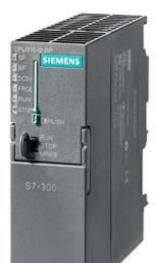
SIPLUS S7-300 CPU 315-2DP -25...+70°C with conformal coating based on 6ES7315-2AH14-0AB0 . Central processing unit with MPI Integr. power supply 24 V DC Work memory 256 KB 2nd interface DP master/ slave Micro Memory Card required
