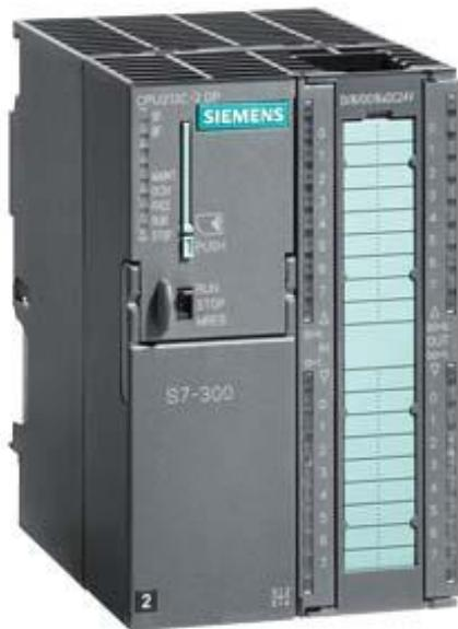
SIPLUS S7-300 CPU 313C-2DP for medial exposure -25...+70°C based on 6ES7313-6CG04-0AB0 . Compact CPU with MPI, 16 DI/16 DO, 3 high-speed counters (30 kHz), integrated DP interface, Integr. power supply 24 V DC, work memory 128 KB, Front connector (1x 40-pole) and Micro Memory Card required
