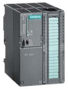
SIPLUS S7-300 CPU 313C-2DP for medial exposure -25...+70°C based on 6ES7313-6CG04-0AB0 . Compact CPU with MPI, 16 DI/16 DO, 3 high-speed counters (30 kHz), integrated DP interface, Integr. power supply 24 V DC, work memory 128 KB, Front connector (1x 40-pole) and Micro Memory Card required
