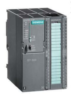
SIPLUS S7-300 CPU CPU 313C-2DP with conformal coating according to EN 50155 T1 Cat 1 Cl A/ B based on 6ES7313-6CG04-0AB0 . Compact CPU with MPI, 16 Dl/16 DO, 3 high-speed counters (30 kHz), integrated DP interface, Integr. power supply 24 V DC, work memory 128 KB, Front connector (1x 40-pole) and Micro Memory Card required
