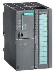
SIPLUS S7-300 CPU 312C with conformal coating according to EN 50155 T1 Cat 1 Cl A/ B based on 6ES7312-5BF04-0AB0 . Compact CPU with MPI, 10 DI/6 DQ, 2 high-speed counters (10 kHz) Integr. power supply 24 V DC, work memory 64 KB, Front connector (1x 40-pole) and Micro Memory Card required
