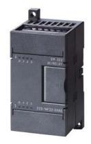
\*\*\*Spare part\*\*\* SIMATIC S7-200, Digital I/O EM 223, only for S7-22X CPU, 32DI 24 V DC, Sink/Source, 32DO 24 V DC; 0.75 A/channel, SOURC
