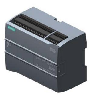
SIPLUS S7-1200 CPU 1215C AC/DC/relay for medial exposure with conformal coating based on 6ES7215-1BG40-0XB0 . compact CPU, AC/DC/relay, onboard I/O: 14 DI 24 V DC 10 DO relay 2 A 2 AI 0-10 V DC 2 AO 0-20 mA DC Power supply: 85-264V AC @ 47-63 Hz, Program/data memory 125 KB
