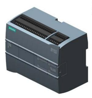
SIPLUS S7-1200 CPU 1215C DC/DC/DC -40...+70°C with conformal coating based on 6ES7215-1AG40-0XB0 . compact CPU, DC/DC/DC, 2 PROFINET ports, onboard I/O: 14 DI 24 V DC 10 DO 24 V DC 0.5 A 2 Al 0-10 V DC, 2 AO 0-20 mA DC, Power supply: DC 20.4-28.8V DC, Program/data memory 125 KB
