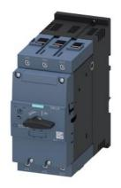
Circuit breaker size S3 for motor protection, CLASS 10 A-release 65...84 A N-release 1170 A screw terminal Increased switching capacity 100 kA
