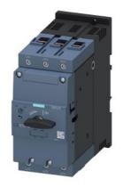
Circuit breaker size S3 for motor protection, CLASS 10 A-release 28...40 A N-release 520 A screw terminal Increased switching capacity 100 kA  $\,$
