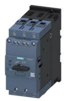
Circuit breaker size S3 for motor protection, CLASS 10 A-release 36...50 A N-release 650 A screw terminal Standard switching capacity with transverse auxiliary switches 1 NO+1 NC  $\,$
