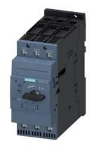
Circuit breaker size S2 for motor protection, CLASS 10 A-release 9.5...14 A N-release 208 A screw terminal increased switching capacity
