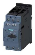
Circuit breaker size S2 for motor protection class 20 A-release 12...17 A N-release 260 A screw terminal Standard switching capacity with transverse auxiliary switch 1 NO+1 NC
