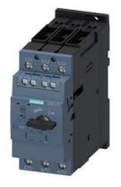
Circuit breaker size S2 for motor protection class 20 A-release 9.5...14 A N-release 208 A screw terminal Standard switching capacity with transverse auxiliary switch 1 NO+1 NC
